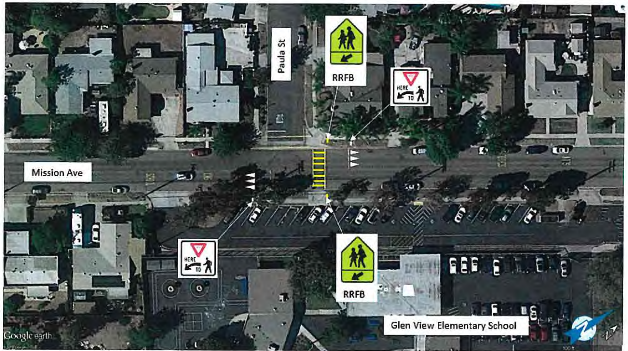
Figure 1–Mid-block Crosswalk Improvements at Glenview Elementary School
