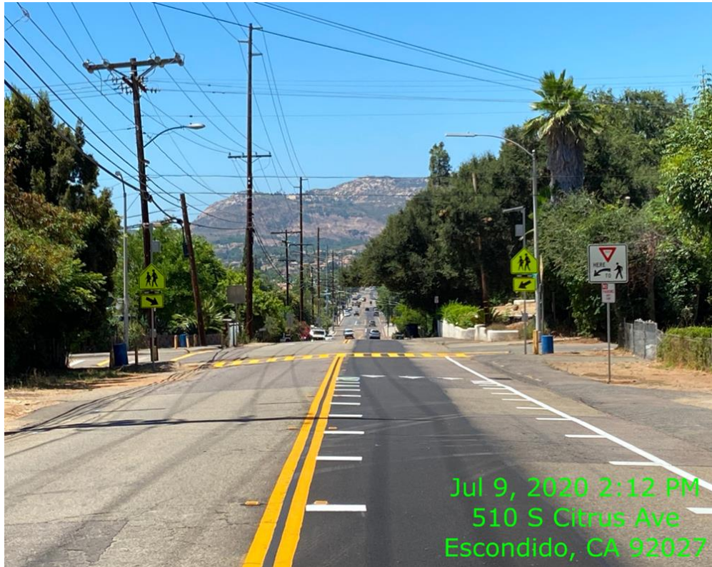
Figure 7: Yield legends now keep vehicles further away from crosswalk and improve visibility of pedestrians.
