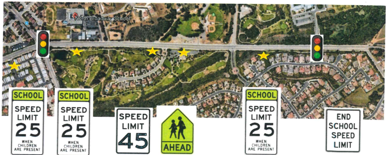
Figure 14: Northbound signage could be refreshed. End School Zone sign could be added end of segment.
