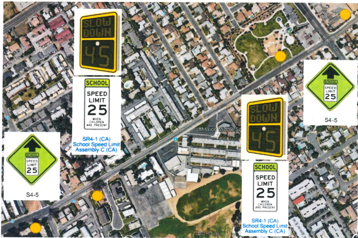
Figure 6: Radar Speed Feedback Signs and approach warning signage could be added.
