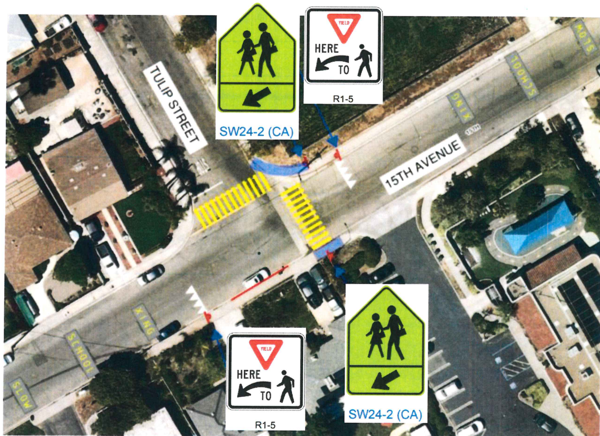
Figure 26: Proposed improvements include a new ramp, signage and markings.
