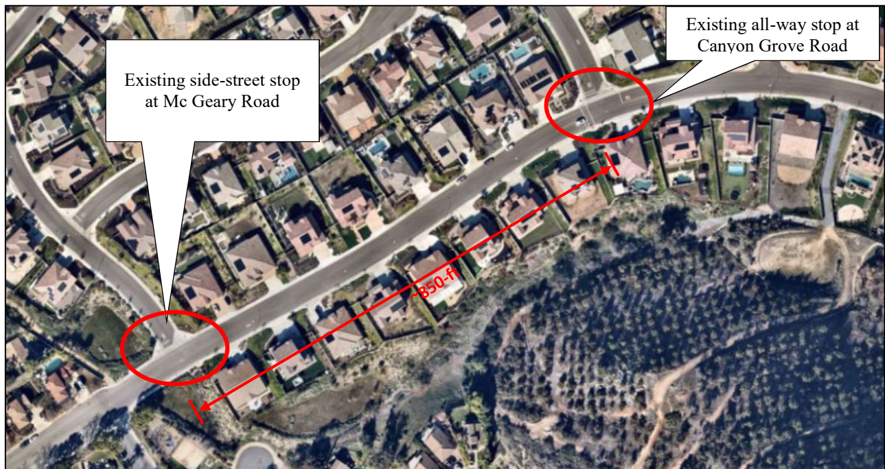
Figure 22: New Stop-controls would work in tandem with the existing All-way Stop at Canyon Grove Road.
